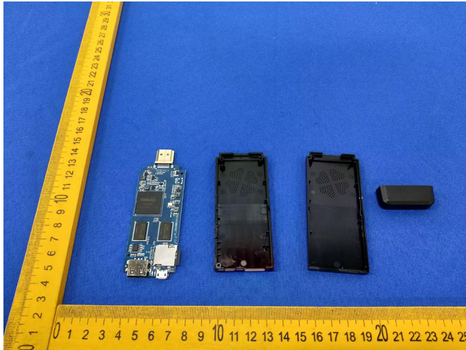
Photo 5 Inside of EUT
