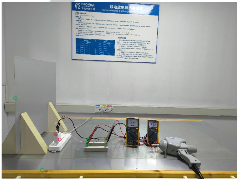
The Photo for Discharge Points of EUT
