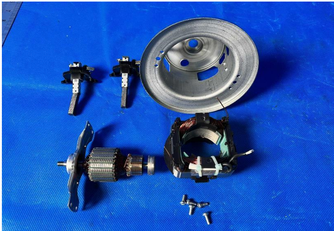
Photo 12 - Internal view of motor V1J-PH22-T
